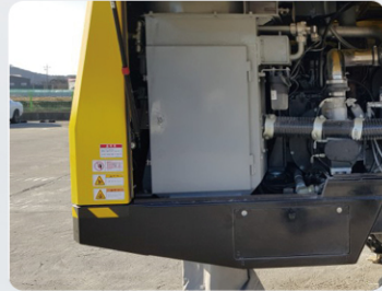
Reliable dust collector with a powerful suction power Suction capacity: over 20~25m 3 /min
